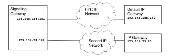
Figure 4 demonstrates the Signaling Gateway configured to exist in multiple IP networks. Example MML for the above configuration is:
